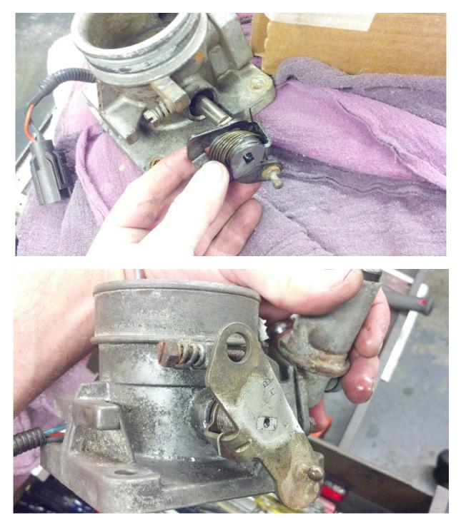
Once the mustang lever is swapped over to the 65mm TB, I drilled and tapped the center of the shaft to secure the lever. I used a drill size #29 and tapped it 8-32x3/8". I used a drop of blue lock-tite and a washer.
