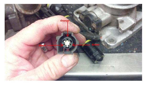
Here you can see the connector was removed from the explorer TPS wiring
