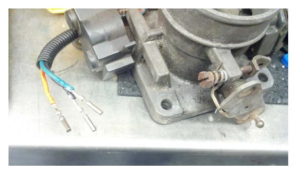
Ready to reinstall pins from explorer TPS into this mustang connector.
