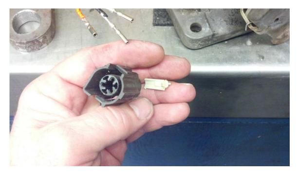
Pins are in, and the center plastic lock is installed...now the TPS is done.
