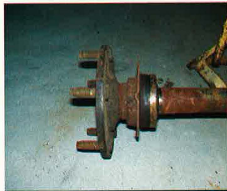
The stock shaft after removal, the studs will need removing, and the drum backing plate should be cut the same size as the retaining plate. Now is a good time to put in new bearings.
