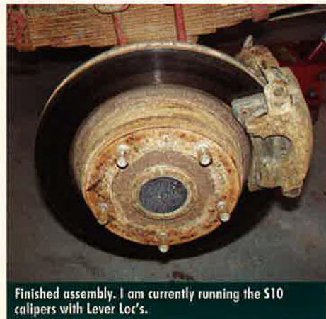
You can see the rotor is mounted behind the axle flange (yes this has been done for some time and I'm due to lube the slide pins).
