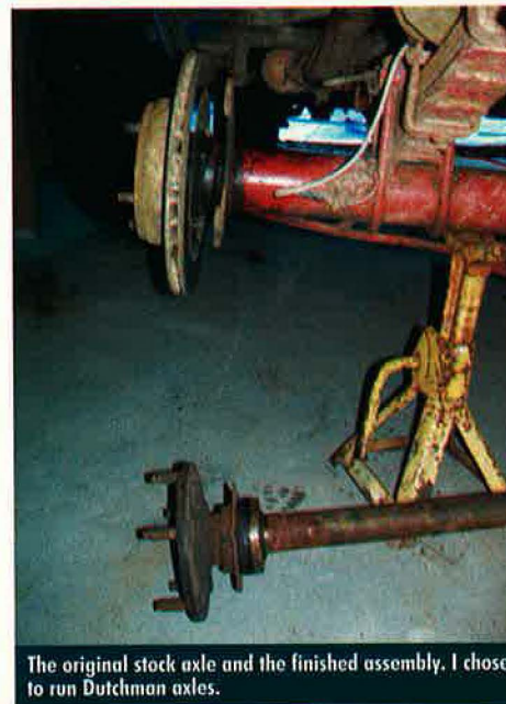
The stock shaft after removal, the studs will need removing, and the drum backing plate should be cut the same size as the retaining plate. Now is a good time to put in new bearings.
