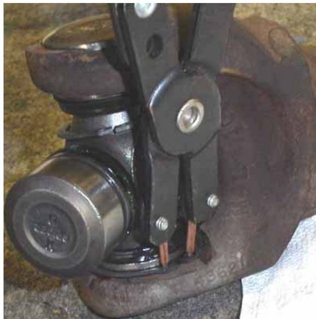
(Snap ring in place in the bearing cap groove to retain it in the yoke)
