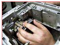
Mike installed the band struts, which will clamp the low/reverse band tight to the low/reverse drum when under hydraulic pressure. After installing the bands, he checked that they were working properly with compressed air (not shown).
