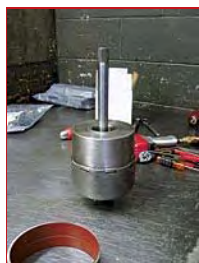
Mike placed the input shaft in the just-completed subassembly.
