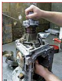
With the trans case standing on end, Mike carefully installed the one-way clutch-equipped output shaft in the governor distributor sleeve.
