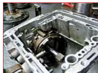
After soaking the low/reverse band in Mercon Transmission Fluid for at least 10 minutes, it was nested over the low/reverse drum.
