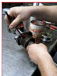
Focusing on the output shaft, Mike installed the governor and applied assembly oil. The output shaft is comprised of governor valves and a distributor.
