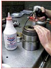
Mike liberally applied Lucas Oil Transmission Fix (LOTF) to all metal surfaces. WTS uses LOTF as an assembly lube--it works really well.
