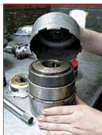
To complete the first subassembly, Mike installed the sun gear, thrust washer No. 5, and the input shell (a.k.a. sun-gear shell).
