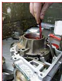
Mike applied LOTF to the governor distributor sleeve, since the opening would be receiving the governor-equipped output shaft, imminently.
