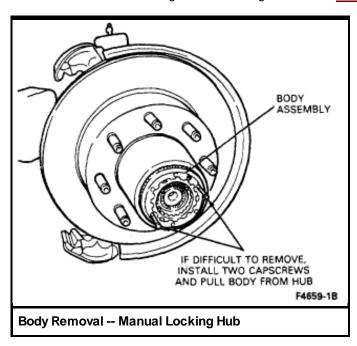
4. Remove the body assembly from the hub. If the body is difficult to remove, install two capscrews and pull the body assembly out of the hub.
