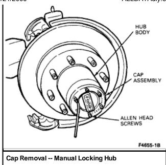
1. Separate the cap assembly from the body assembly by removing six capscrews and remove the cap from the body.
