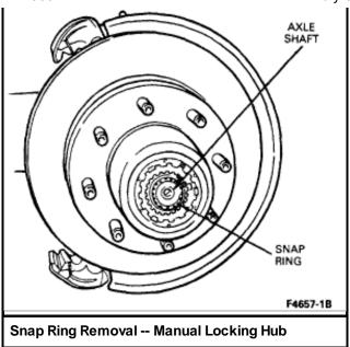
3. Remove the lock ring seated in the groove of the wheel hub.
