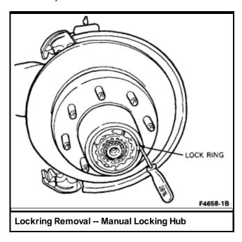
2. Remove the snap ring that retains the axle shaft in the hub body assembly.
